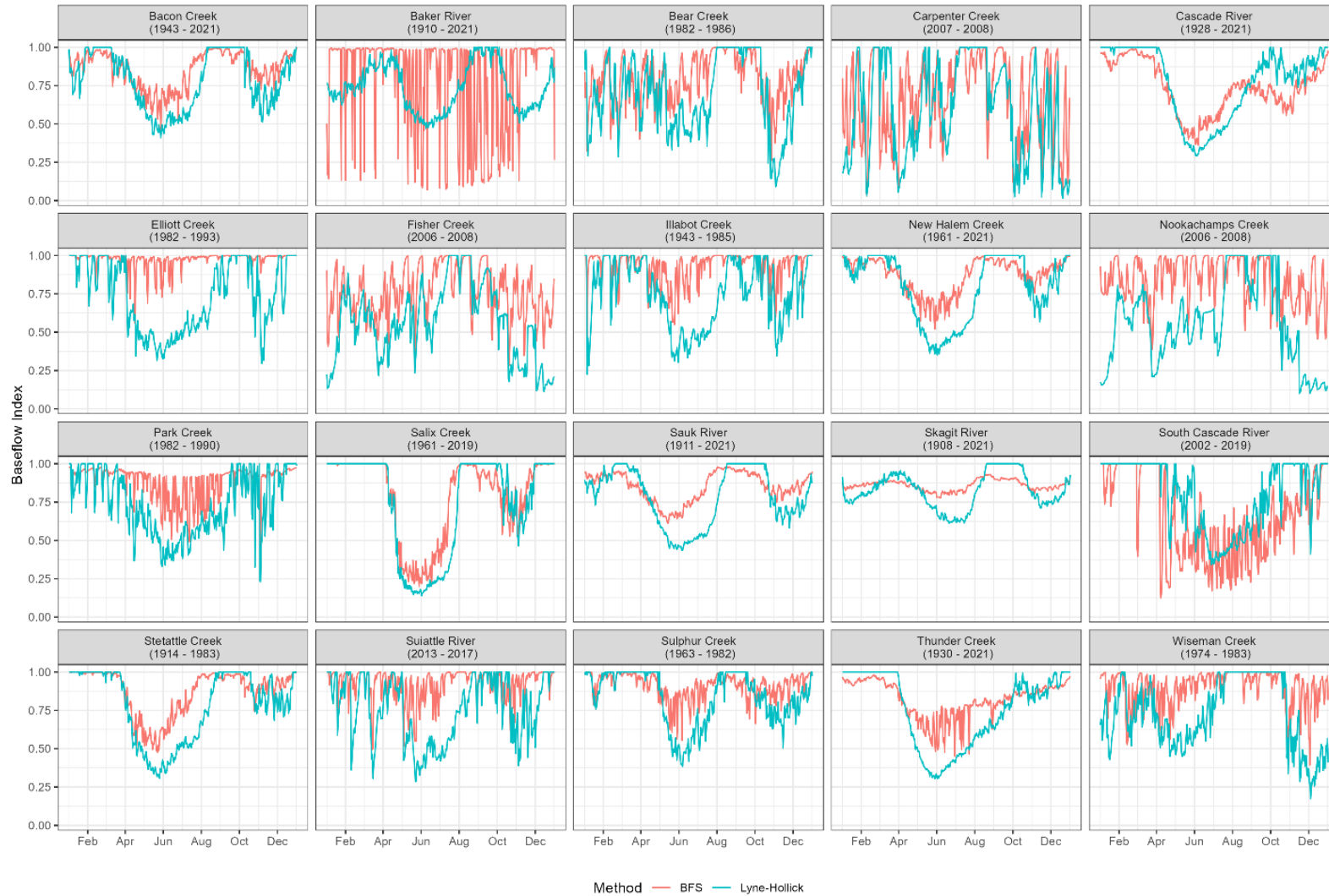
Figure 4. Median daily BFI method comparison by stream including all gages and all years (the Lyne-Hollick method alpha parameter value equals 0.98).
