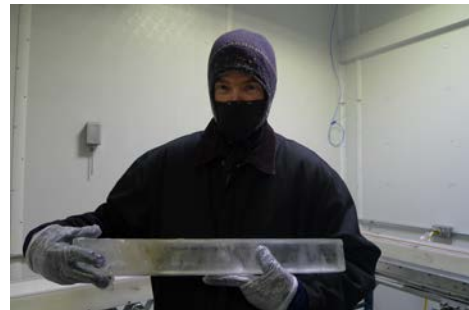
Figure 5: MS student Dan Pittenger identifies a dust layer in a section of the South Cascade ice core.
